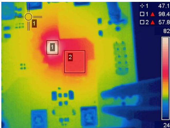
Figure 21: Thermal Image at VIN = 12V, IOUT = 12A (IR3476: 98°C, Inductor: 58°C, PCB: 47°C)
